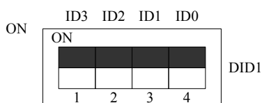
The above chart shows "1111", so it means that the physical ID is 15.
